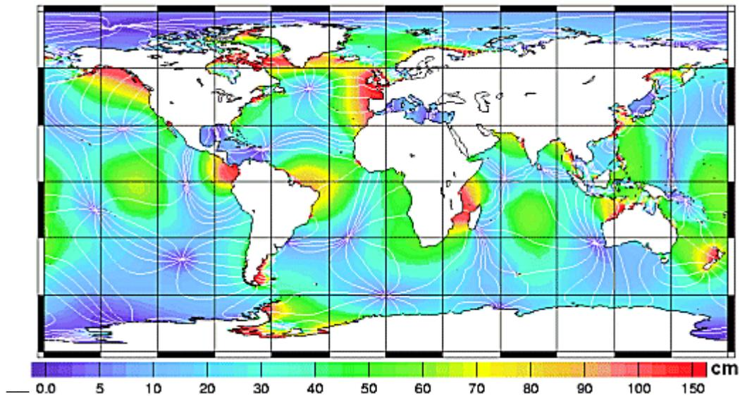
Figure 6.16. Amplitude of the M2 tidal constituent (in centimetres) derived from the FES99 model. Cotidal lines indicating the phase every 30 degrees originate at amphidromic points where the tidal range is zero. (Credits Legos/CNRS)
