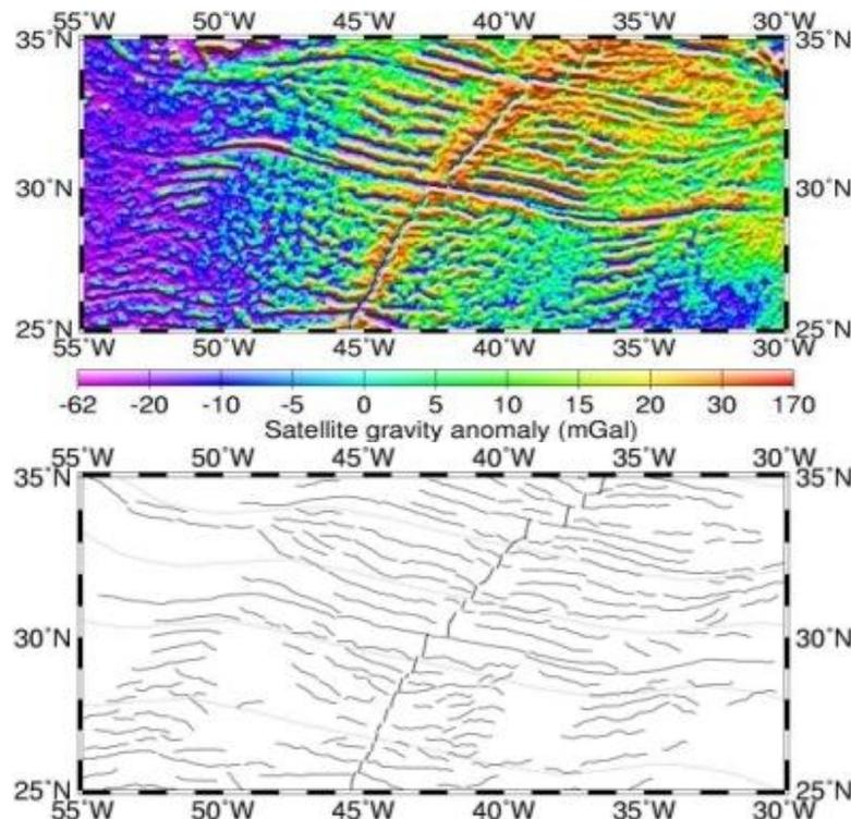
*Figure 6.8.* Gravity anomalies (top) in the North Atlantic measured in milligals ( $1 \text{ mGal} = 10^{-5} \text{ m/s}^2$ ). Since gravity depends on distribution and density of material, features such as the Mid-Atlantic Ridge and fracture zones show up clearly (Credits [Legos](#)).
