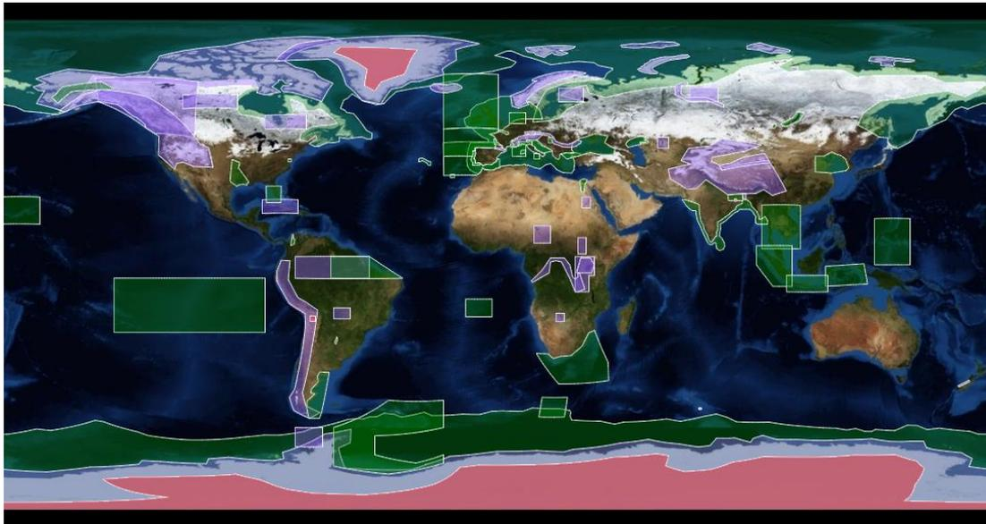
Figure 5.55. CryoSat-2 mode mask. SAR (green), SARin (purple) and LRM (red and others) operating modes. Credit: ESA
