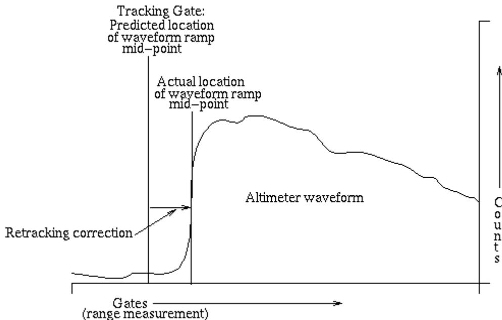
*Figure 5.44. Typical ice sheet altimeter waveform illustrating the retracking correction that must be applied to compensate for deviation of the waveform's leading edge from the on-board altimeter tracking gate. (Credits NASA/GSFC)*
