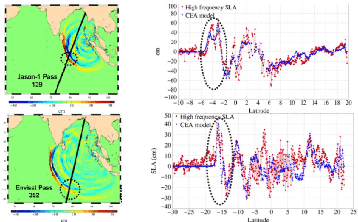
Figure 6.9. Ground track for Jason-1 (top left) and Envisat (bottom left) overlaid by the CEA wave propagation simulation at the time of the satellite's passage. The area corresponding to the tsunami's front is circled. Sea level anomalies measured by Jason-1 and Envisat compared to the CEA simulation (top and bottom right) (Credits [CEA](#) & [CLS](#)).
