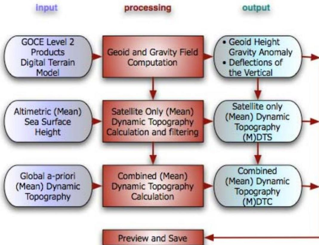
Figure 5.40. GOCE User Toolbox Workflow (Credits DTU)
