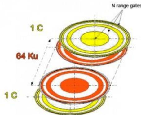
Figure 5.58. LRM Resolution Cell (Credit: TAS-F)
