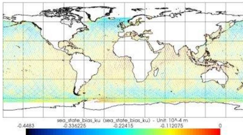
Figure 5.36. Amplitude in metres of the sea state bias correction computed from empirical model for the Ku-band, here for the Jason-1 cycle 223. This map is drawn using the BRAT from the Jason-1 GDR products.
