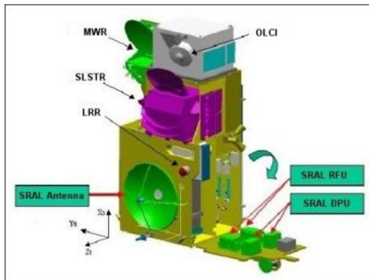
Figure 7.91. Conceptual view of SRAL altimeter on Sentinel-3 (Credits [ESA](#))
