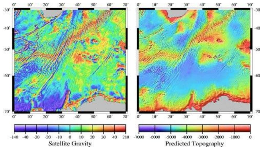
Figure 6.4. Gravity anomalies (left), derived from altimetry, and predicted topography (right) deduced from these gravity anomalies plus in situ measurements. (Credits [NOAA/Scripps Institution of Oceanography](#))
