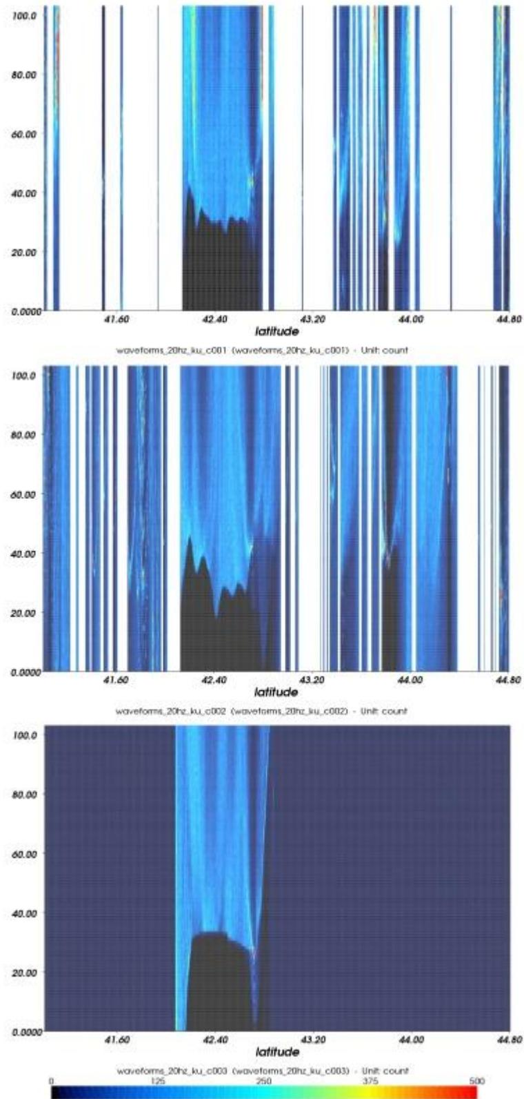
Figure 6.113. Set of juxtaposed waveforms as a function of latitude ( $41^{\circ}\text{N} - 45^{\circ}\text{N}$ , pass #131) and as seen from above for the first three cycles of OSTM/Jason-2. Each cycle corresponds to a different tracker: SGT for cycle 001, Median tracker for cycle 002 and Diode+MNT for cycle 003
