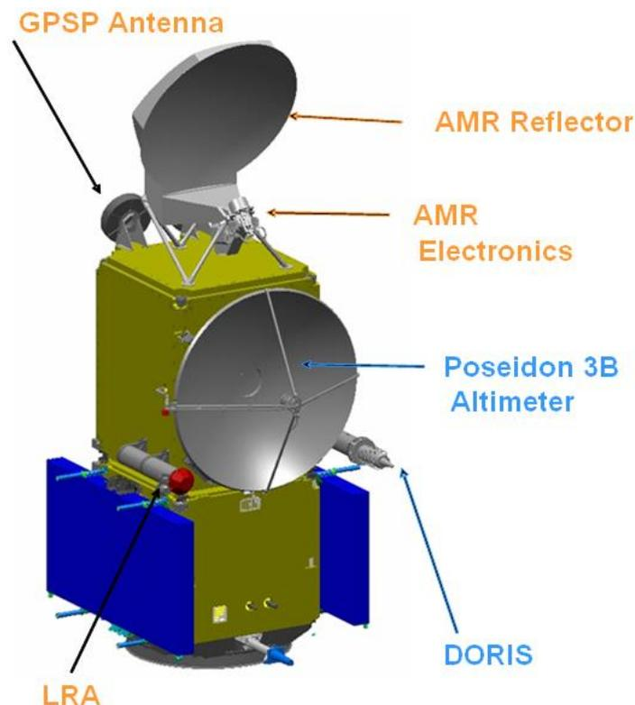
Figure 7.87. Jason-3 instruments
