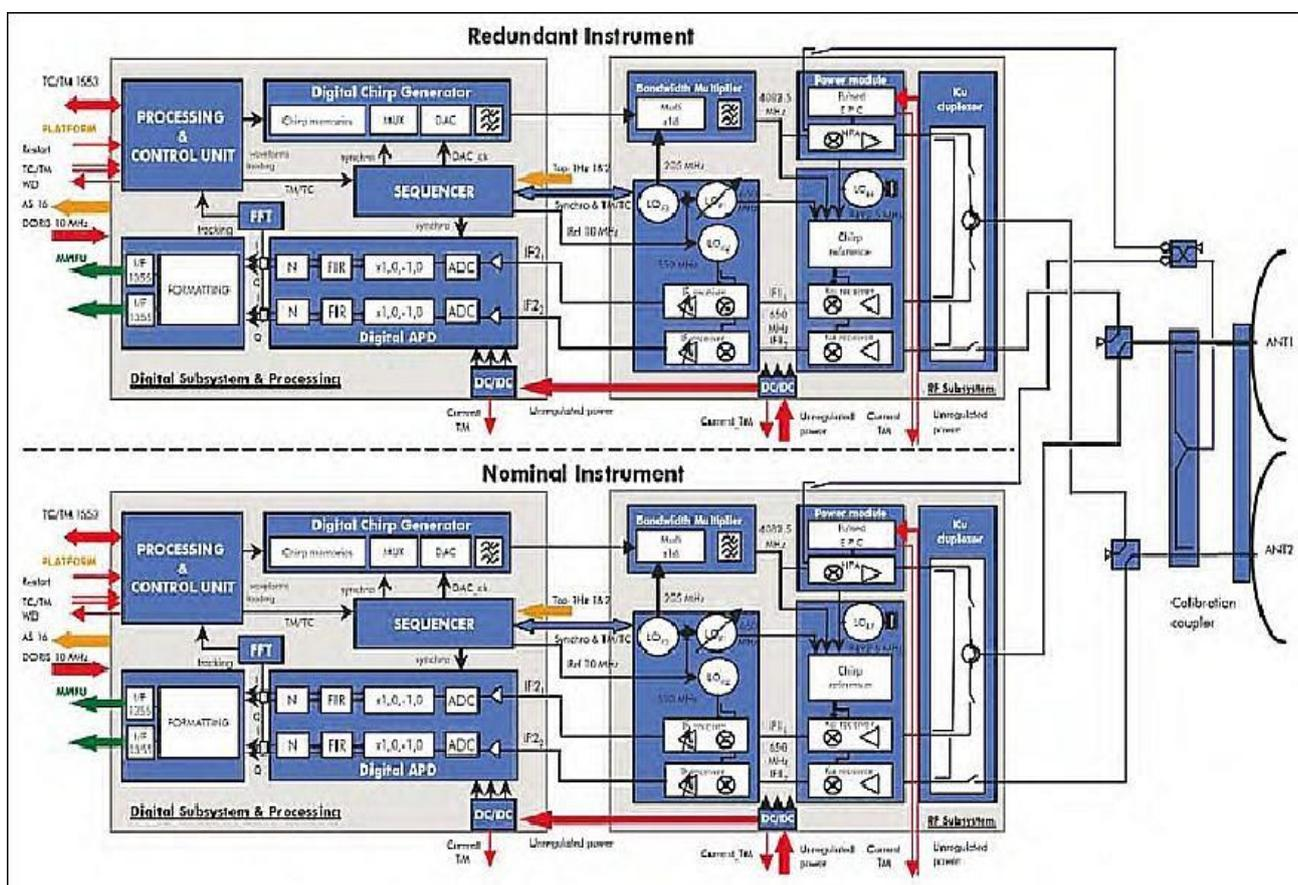
Figure 5.51. Block diagram of the SIRAL instrument. Credit: ESA
