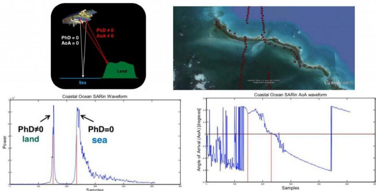
*Figure 6.60. Off nadir returns in SARin mode. (Top left) Schematic of the geometry of a nadir ocean and off nadir land echo. (Top Right), Examples of non-nadir echoes received on pass close to Cuba, with true echoing locations identified. (Bottom Left) Power waveform, showing land echo received before ocean echo, and (Bottom right) phase waveform. The two red lines identify the position of the first echoes from the land and ocean reflectors.*
