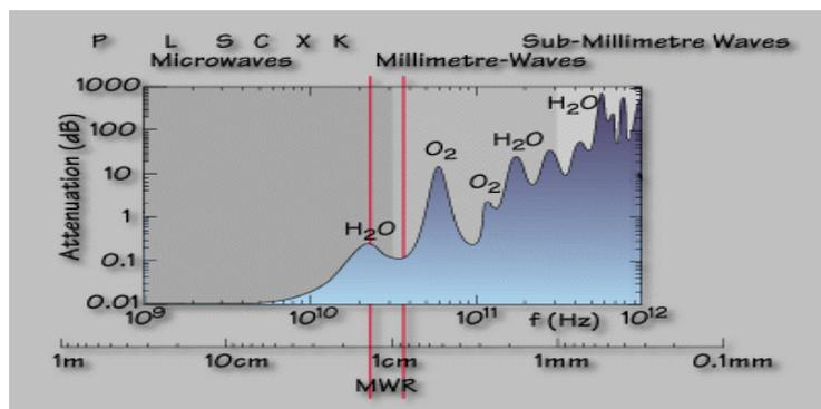
Figure 7.34. Electromagnetic spectrum and MWR frequencies
