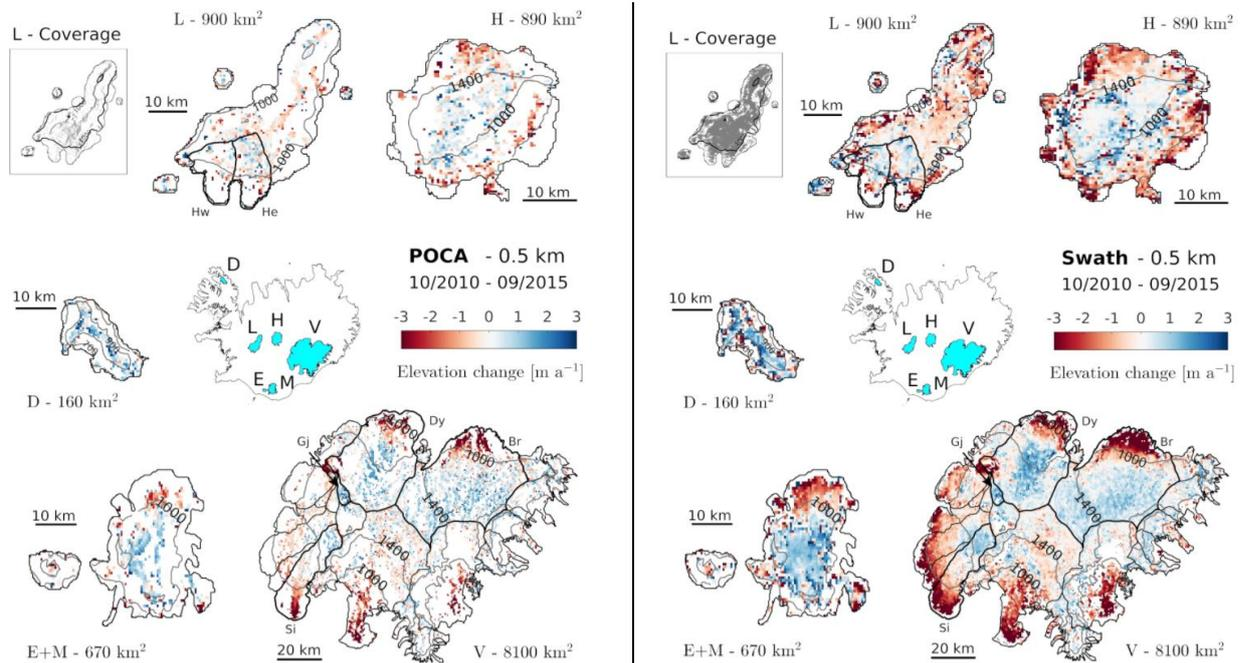
Figure 6.26. Comparison between swath-processed (Swath) and conventional (POCA) surface elevation change rates over the six largest ice caps in Iceland, representing 90% of the glaciated area. V (Vatnajökull), L (Langjökull), H (Hofsjökull), M (Mýrdalsjökull), D (Drangajökull), and E (Eyjafjallajökull). The inset shows the location of individual elevation measurements by using Swath and POCA approaches over Langjökull. [Credit: Luca Foresta et al. (2016).]
