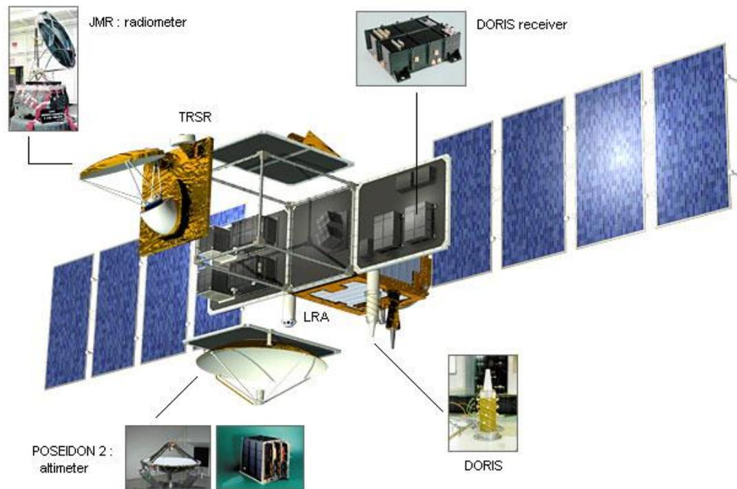
Figure 7.43. Jason 1 instruments
