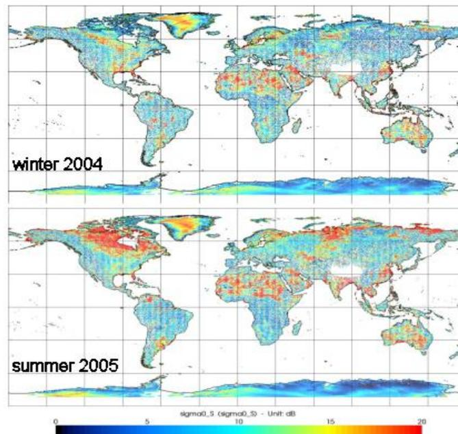
Figure 6.111. Backscatter coefficient  $\Sigma_0-S$  from ICE-2 retracker for Envisat cycle 034 (top) and 040 (bottom): several river basins such as Orinoco, Mississippi, Amazon, Parana, Lena, etc, and areas with melting snow during boreal summer are clearly visible.
