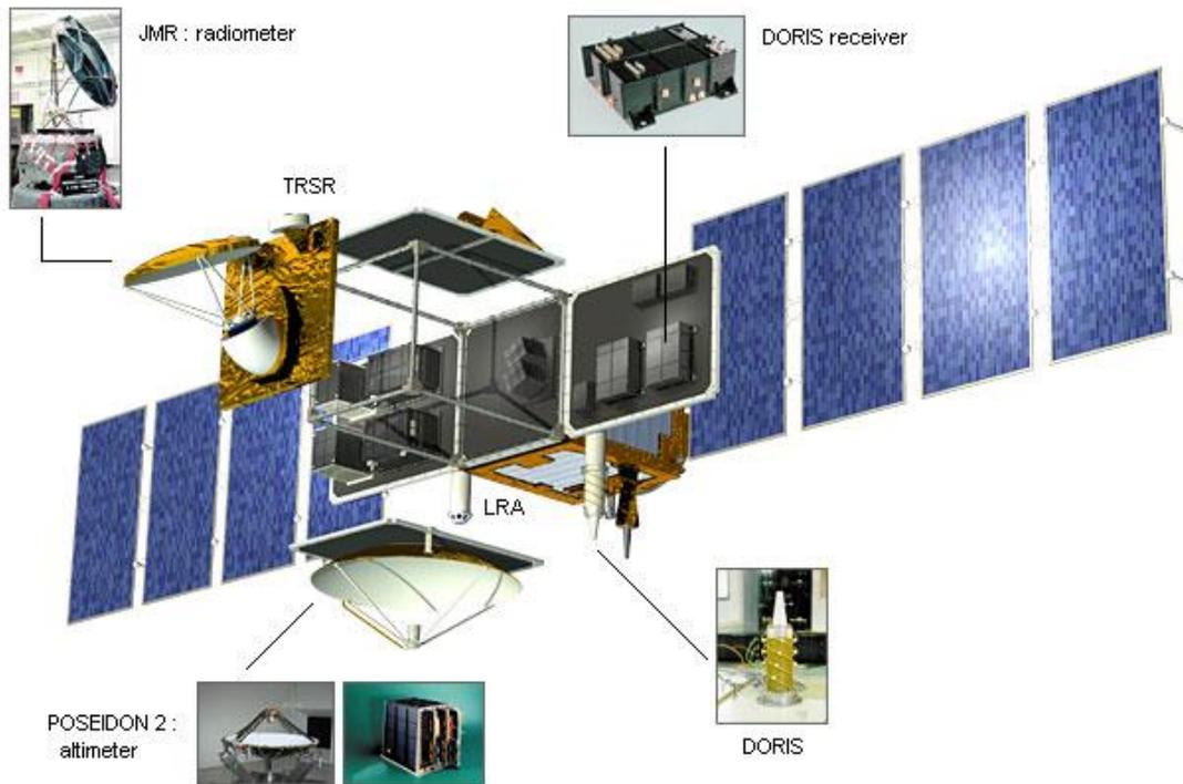
Figure 7.63. Jason 2 instruments
