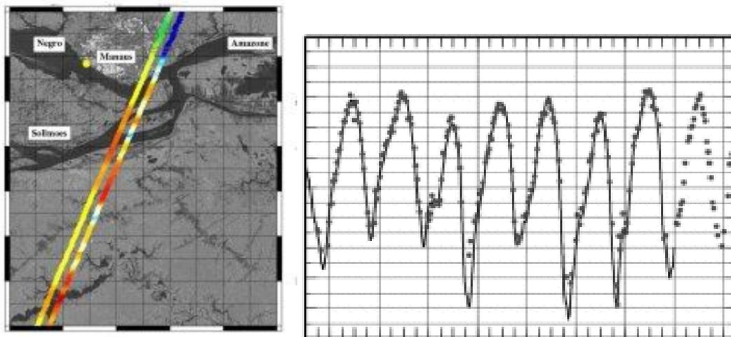
*Figure 6.105. Right: Water level time series in the Amazon for T/P track 63 (3.21°S-3.14°S), in metres; dots represent in situ data from the Manau station. Left: Overview of the geographic window showing the stations; the backscatter coefficient and measurement density parameter have been computed along T/P track 63.*
