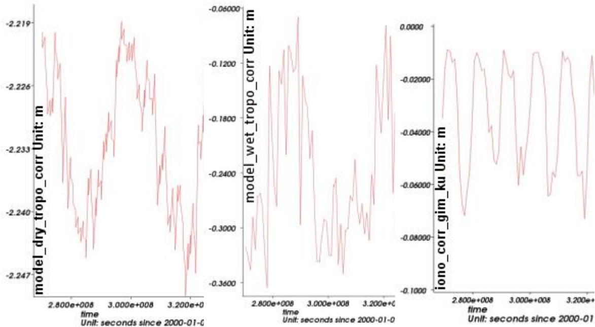
*Figure 6.119. Amplitudes in metres of the dry tropospheric correction derived from model (left), of the wet tropospheric correction derived from model (middle) and of the ionospheric correction derived from the GIM model (right).*
