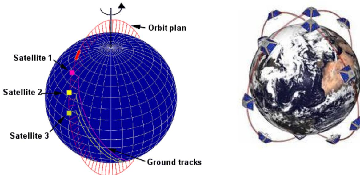
*Figure 5.49. The WITTEX (Water Inclination Topography and Technology Experiment) altimetry satellite constellation project. (Credits John Hopkins University Applied Physics Laboratory) and GANDER (Global Altimeter Network Designed to Evaluate Risk) constellation of microsats in 2 orbit planes (SSTL)*
