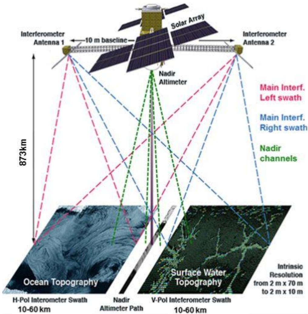
Figure 7.95 SWOT Dual-swath Ka-band radar interferometry system. (Credit: CNES/JPL)
