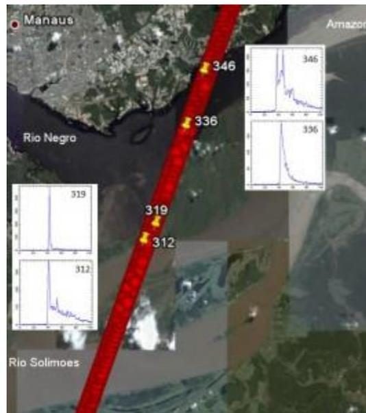
Figure 5.13. Jason-2 waveforms on Amazon river: specular waveform (n°319) result of the return signal from very reflective surfaces like water bodies, multi peaked waveforms result of heterogeneous targets in the footprint.
