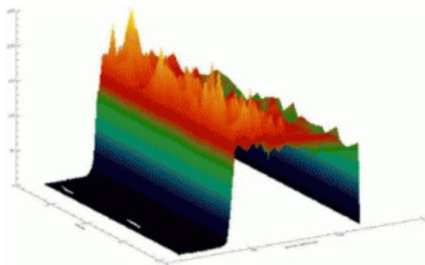
Figure 5.4. Poseidon-2 (Jason-1 altimeter) first waveforms. (Credits CNES)
