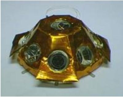
The LRA is an array of mirrors that provide a target for laser tracking measurements from the ground. By analysing the round-trip time of the laser beam, we can locate very precisely where the satellite is on its orbit.
