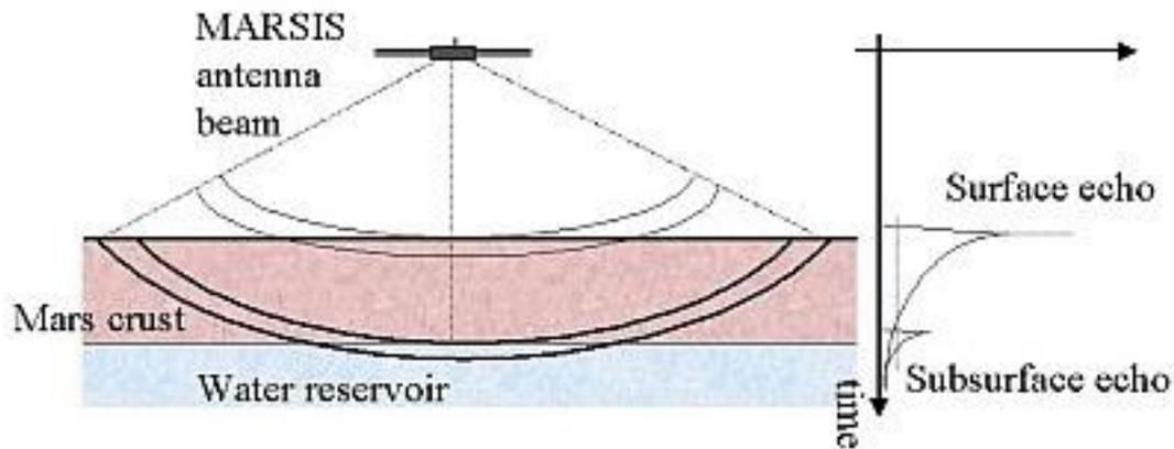
Figure 7.98. MARSIS Principle of Operation (Credits ESA)
