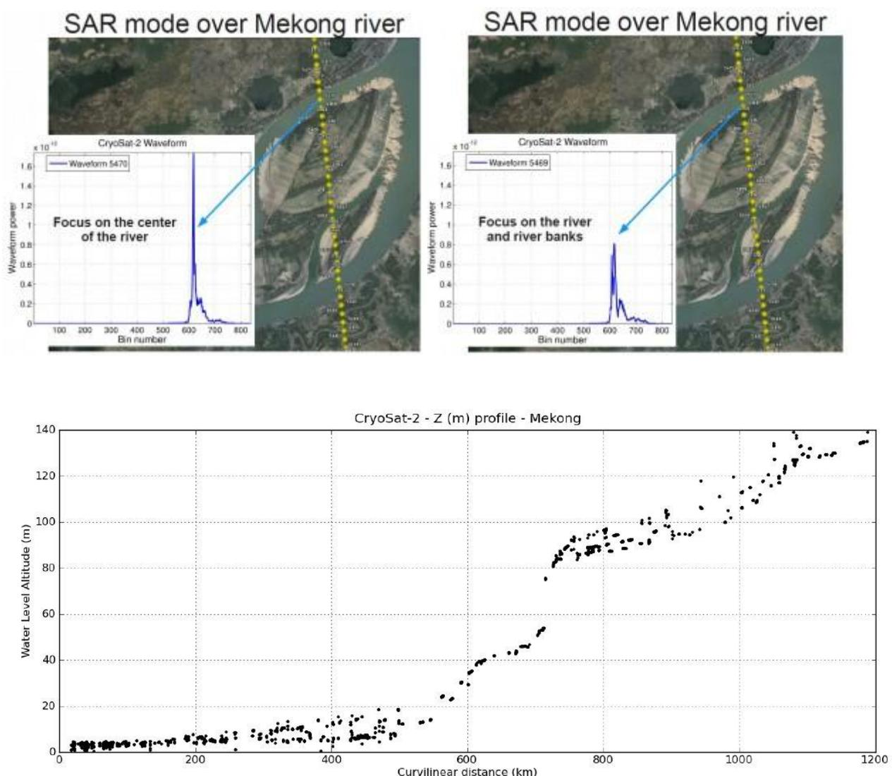
Figure 6.53. Illustration of SAR waveforms over the Mekong river, left and river profile compute from SAR data, Bercher et. al.
