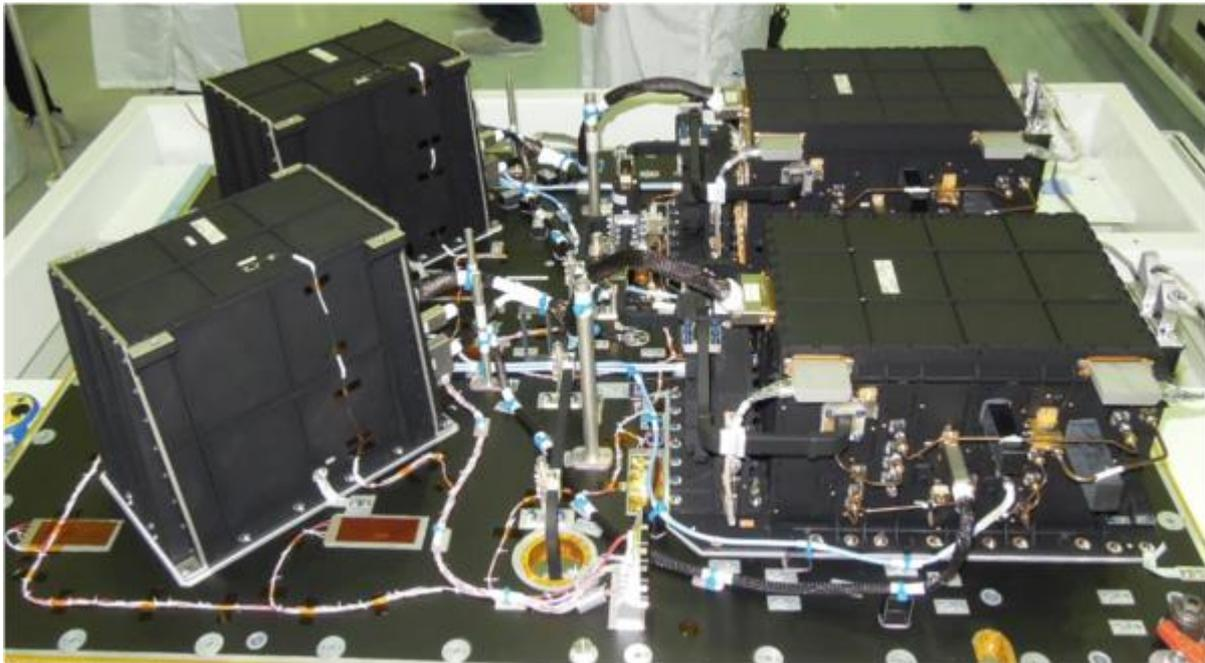
Figure 7.88. Poseidon-3B being integrated on Jason-3 (Credits CNES)
