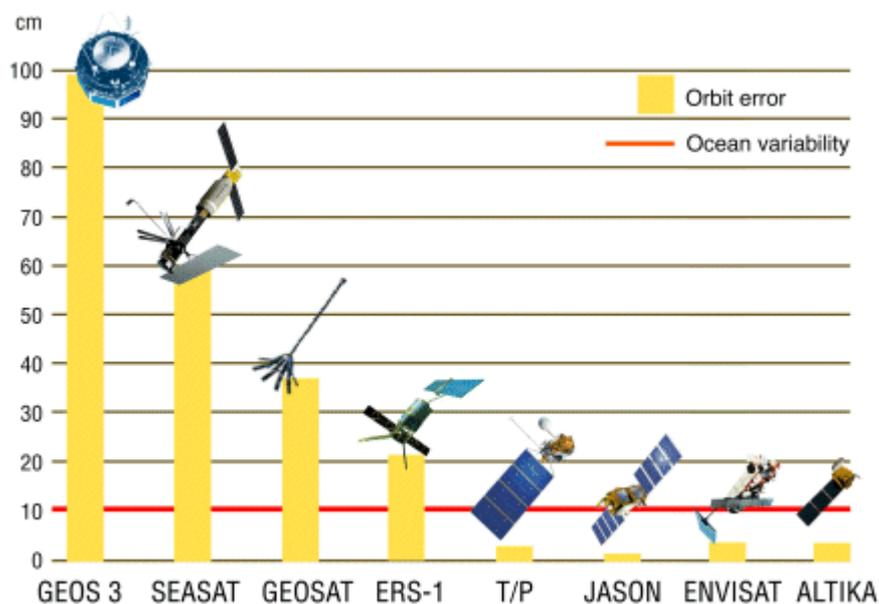
*Figure 7.1. Improvements in measurement accuracy since the first satellite altimetry missions has enabled us to observe ocean variations at close quarters since 1992. (Credits [CNES](#))*
