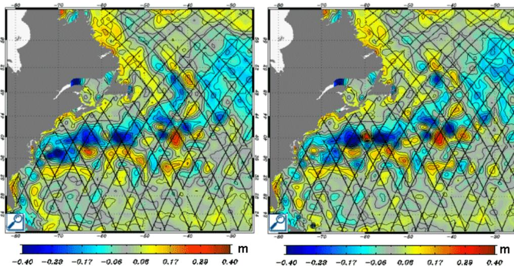
Figure 6.15. Sea level anomalies on 8 January 2003 from the medium-resolution Mercator model ( $1/3^\circ$ ), with assimilation of in situ SST measurements and (left) Jason-1 data only, (right) all available altimetry satellite data (Jason-1, ERS-2 and GFO). More detail can be seen in the right-hand figure (Credits Mercator Ocean).
